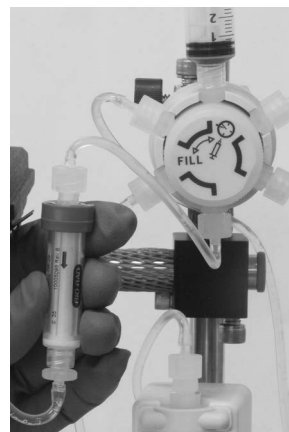
Figure 7.10. MV-6 in Sample Load position, turned as far left as possible.
