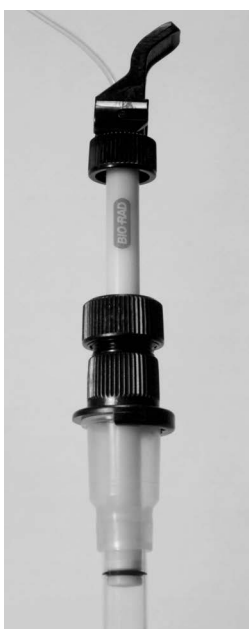
Figure 6.5. Adjusting the O-ring. Cam latch in position 1. White flow adaptor in the glass column.
