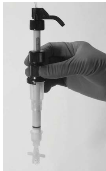
Figure 6.13. Closing the cam latch, position 3.
