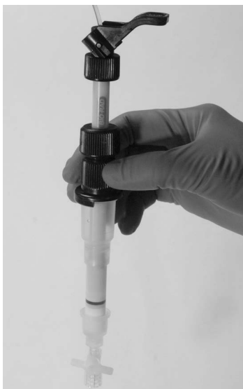
Figure 6.12. Adjusting the flow adaptor height to the resin bed. The cam lock is moved to position 2. The syringe is removed from the tubing and the tubing is placed into the beaker. The two-way stopcock is moved to the closed position. The flow adaptor has been fully lowered to just above the resin bed. The lowering of the flow adaptor body should force the excess buffer out of the flexible tubing into the beaker.
