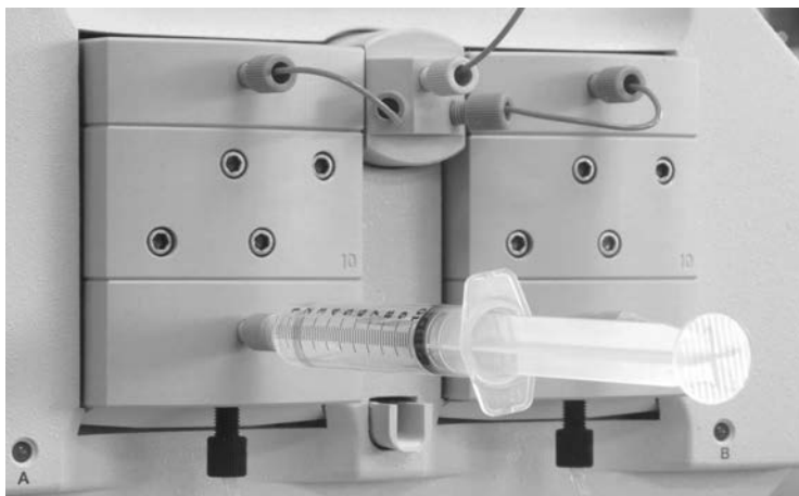
Figure 8.3. Priming the workstation pumps. A complete pump head on the DuoFlow system is shown here. Priming pump: A syringe is used to draw fluid into the inlet tubing for Pump A and Pump B. The pumps cannot pull fluid into the lines if there is air in the lines. Priming also serves to remove any air bubbles from the lines that could damage columns further downstream.
