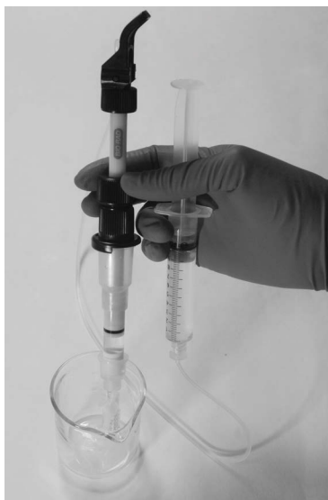
Figure 6.11. Inserting the flow adaptor into the column packed with resin. The cam latch is in position 1 and the flow adaptor has been inserted into the column to the top of the water above the resin. The two-way stopcock at the bottom of the column is open to allow buffer to drain out as the flow adaptor is lowered. The syringe is still attached to the tubing since this prevents water from flowing back up into the syringe at this time.
