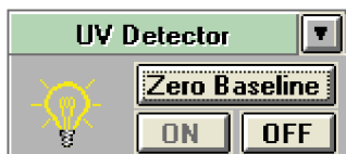
Figure 8.8. Manual control of the UV detector. The UV lamp automatically turns on when you turn on power to the workstation. The UV lamp can be turned on and off by clicking the On and Off buttons from the UV detector control panel on the Manual screen.
