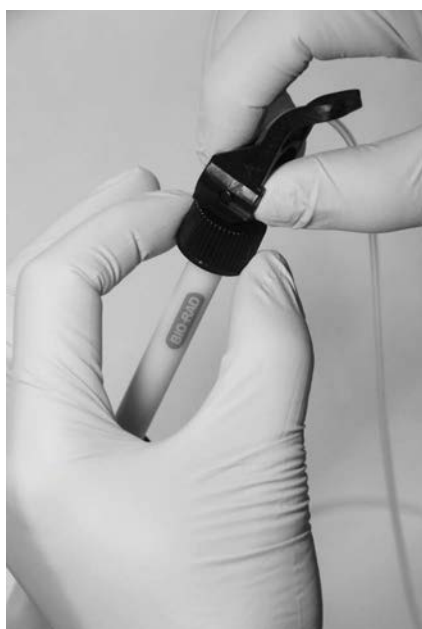
Figure 6.7. Final adjustment of the tension on the O-ring. While holding the cam base with one hand, the cam latch is turned clockwise to tighten the o-ring and turned counterclockwise \frac{1}{4} turn to loosen the O-ring enough to remove the flow adaptor to add resin to the column.
