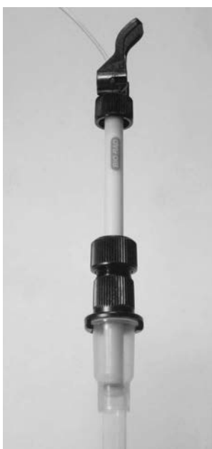
Figure 6.6. Adjusting the tension on the O-ring if the flow adaptor will not slide into the column. The flow adaptor cannot slide beyond the yellow plastic flange due to the O-ring not fitting. While holding the cam base with one hand, the cam latch is turned counterclockwise to loosen the O-ring. (Figure 6.7) White flow adaptor in the column. (Figure 6.5)
