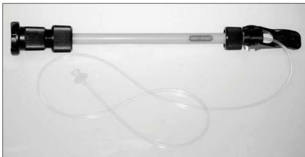
Figure 6.3. Preparing the flow adaptor to be fit into a glass Econo-Column column.
