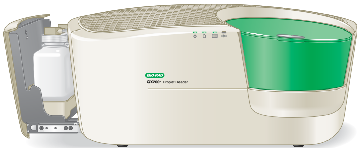
Fig. 26. Replacing droplet reader oil and removing waste. Slide out the carriage containing the droplet reader oil and waste receptacles to remove and replace the bottles (left). After replacing oil, click Prime to fill the lines; other instrument maintenance routines are for use by field specialists only.
