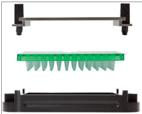
Figure 3-1: Placing the 96-well plate into the plate holder
